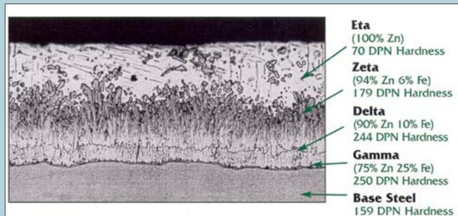
Figure 4: Photomicrograph of a Galvanized Coating
