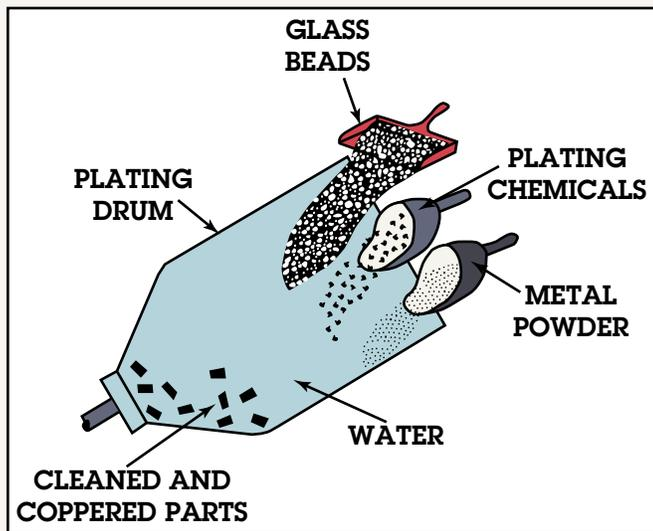
Figure 7: Mechanical Plating
