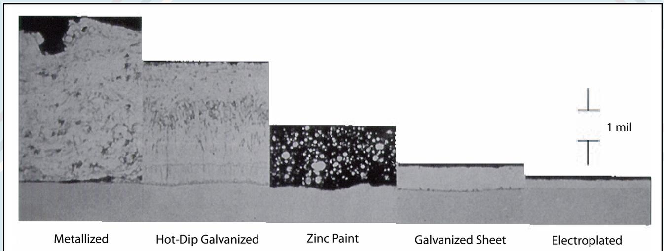
Figure 2: Microstructures of Various Zinc Coatings
