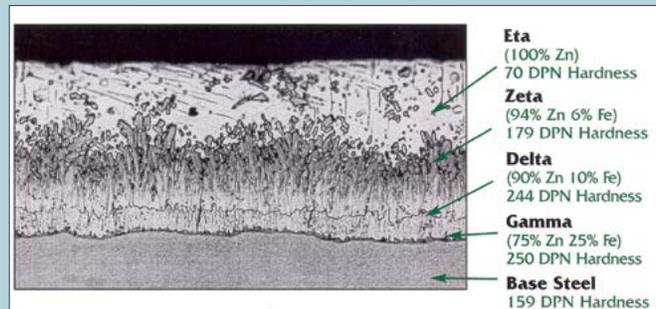
Figure 4: Photomicrograph of a Galvanized Coating
