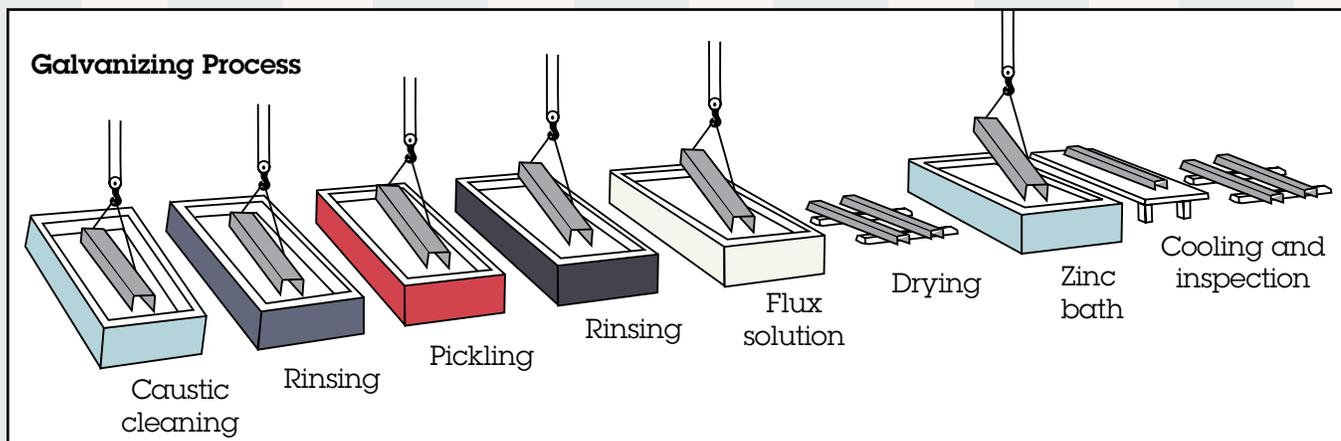
Figure 3: Batch hot-dip galvanizing processes
