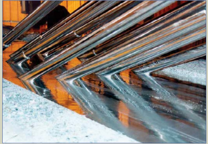
When steel is hot-dip galvanized, zinc - a 100% recyclable natural element - can provide superior barrier and cathodic corrosion protection.
