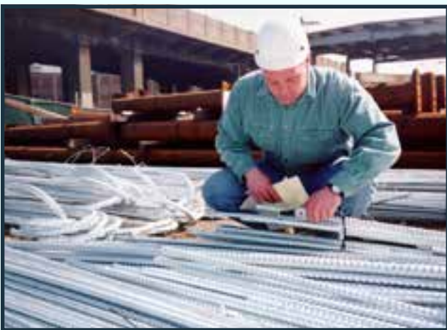
Inspection of galvanized rebar
