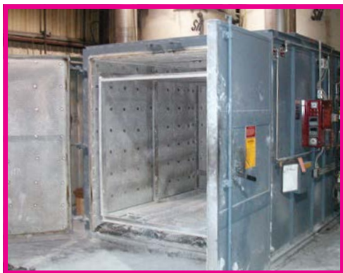
Ovens are used to bake galvanized steel prior to powder coating to prevent outgassing.
