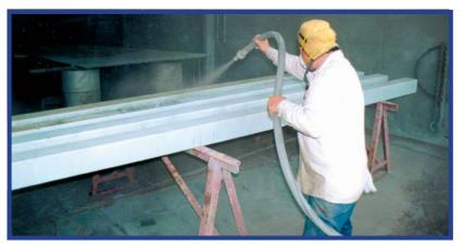
**Sweep blasting** is the preferred method of profiling because of the soft nature of the zinc surface.
