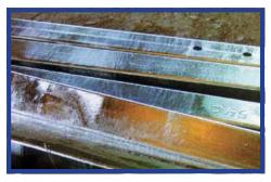
**Newly galvanized steel,** seen above, only requires grinding drips and runs flat and a rinse/ dry prior to painting.
