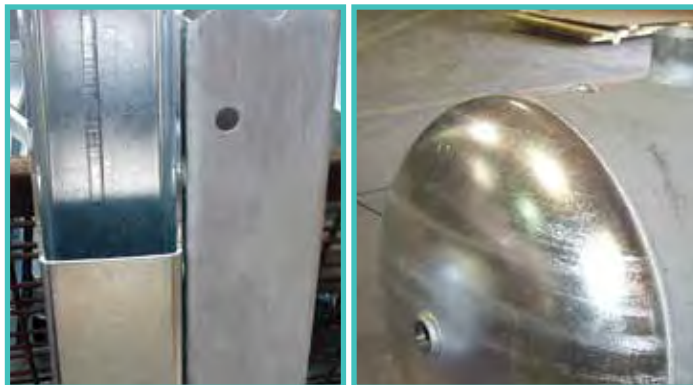
FIGURE 9: SHINY VS. DULL (ACCEPTABLE)
