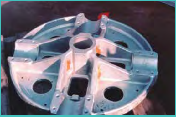
FIGURE 29: SAND EMBEDDED IN CASTING (REJECTABLE)
