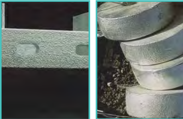
FIGURE 26: ROUGH SURFACE CONDITION/ STEEL SURFACE CONDITION (ACCEPTABLE)
