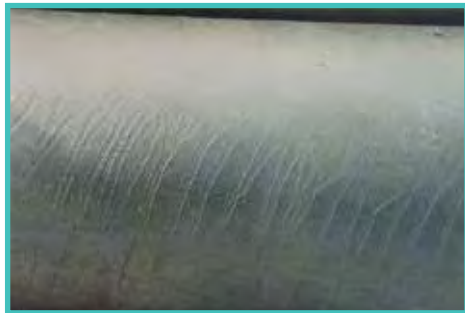
FIGURE 31: FISH BONING (ACCEPTABLE)
