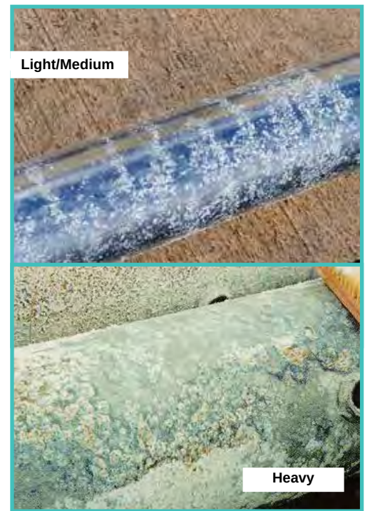
FIGURE 36: WET STORAGE STAIN (LIGHT (1) OR MEDIUM (2) IS ACCEPTABLE, HEAVY (3) IS REJECTABLE)
