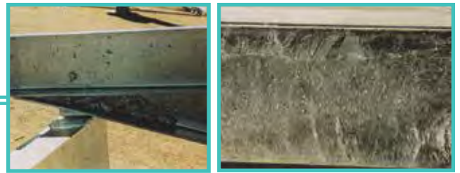
FIGURE 19: DROSS INCLUSIONS (ACCEPTABLE UNLESS LARGE, AND IF REMOVED, A BARE SPOT IS EXPOSED)
