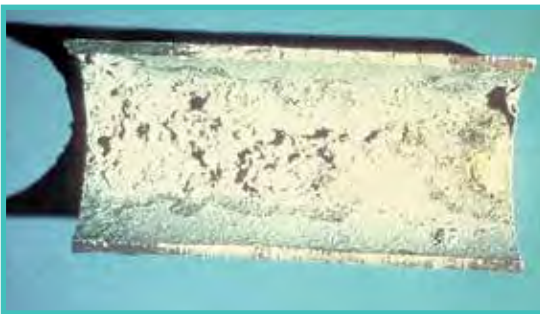
FIGURE 22: FLUX INCLUSIONS FROM INTERIOR OF PIPE (REJECTABLE)
