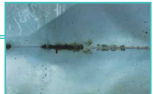
FIGURE 37: ZINC SKIMMINGS (ACCEPTABLE)
