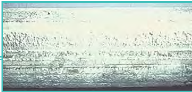
FIGURE 8: ROUGH COATING DUE TO PHOSPHOROUS LEVELS OVER 0.04% (ACCEPTABLE UNLESS HANDRAIL)
