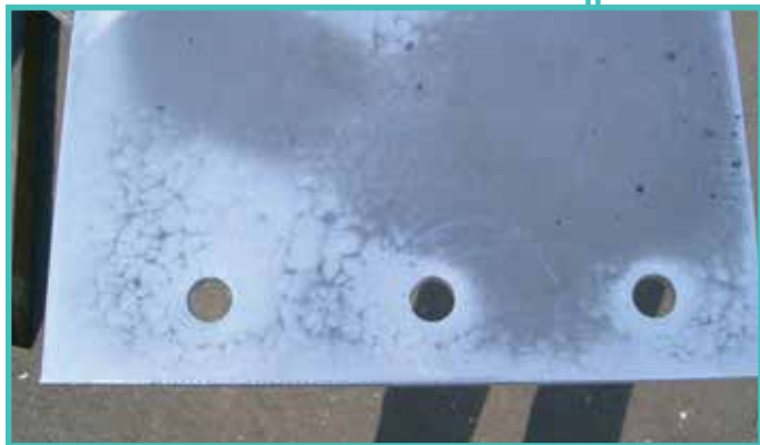
FIGURE 10: GRAY COATING DUE TO UNEVEN COOLING RATE (ACCEPTABLE)
