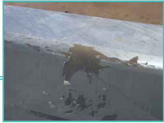
FIGURE 16: DELAMINATION (ACCEPTABLE IF MINIMUM THICKNESS LEVELS ARE MET)
