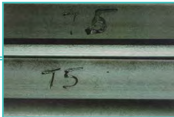
FIGURE 32: SURFACE CONTAMINANT (REJECTABLE)
