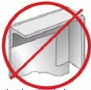
Figure 13: Avoid uneven thickness at joints
