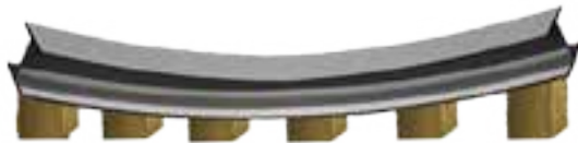
Figure 19: To support a camber beam, lay the product on the strong axis and support with as many blocks as possible.
