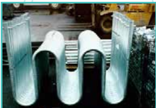
Figure 5: Excessive cold working can result in strain-age embrittlement
