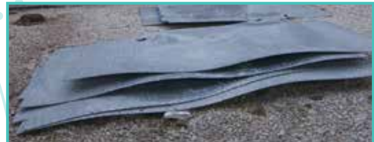
Thin sheets that warped during the galvanizing process
