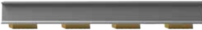
Figure 18: Products should be laid flat after galvanizing. Additional supports should be added along mid-sections as required to prevent sagging.
