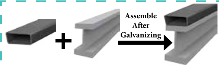
Figure 9: Fabricate and galvanize individual part as separate loose items and then assemble after galvanizing.
