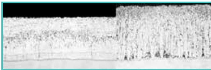
Figure 4: Recommended Silicon (left) vs Reactive Steel (right) (not to scale)
