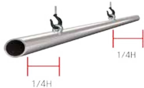
Figure 22: Lift points for galvanizing should be located at quarter points along the product length.
