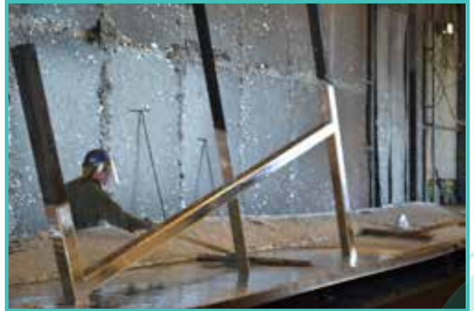
Figure 17: Avoid leaving the mid portion of long and slender products unsupported as sagging can introduce a permanent bow.
