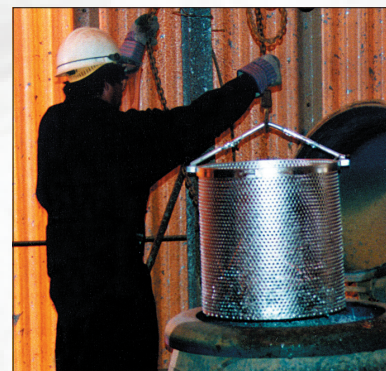
Fasteners in perforated basket are removed after being spun to remove excess zinc.
