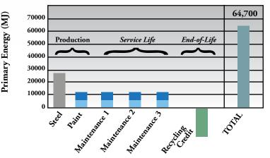
Figure 11: Life-Cycle Energy: HDG vs. Paint
