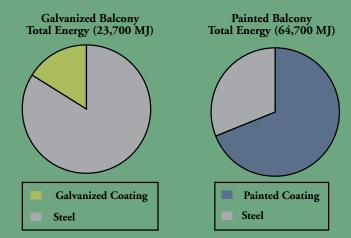
Figure 12: Coating Energy Consumption: HDG vs. Paint
