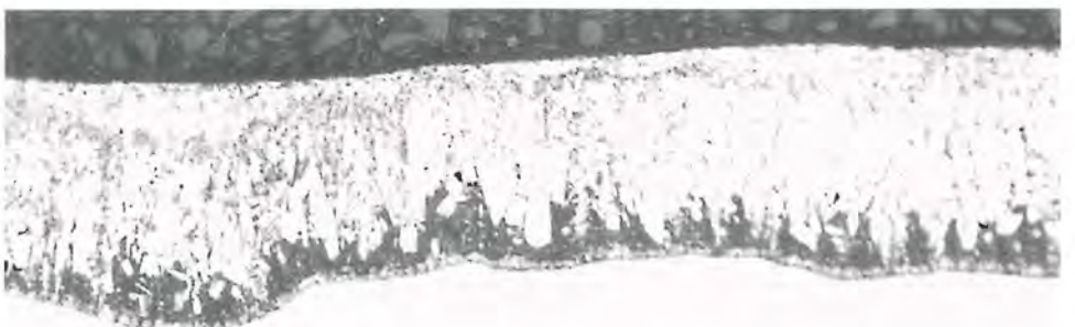
3b. Cross section of a Hyper- Sandelin coating
