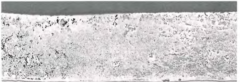
3a. Cross section of a Sandelin coating.
