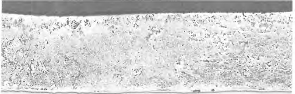
12. Coating on a 'classical' Sandelin steel with low phosphorus.
