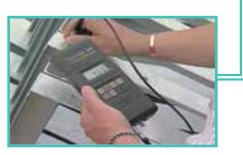
FIGURE 4: DIGITAL THICKNESS GAUGE
