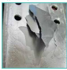
FIGURE 21: FLAKING (REJECTABLE)
