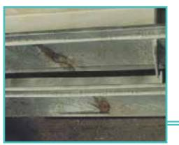
FIGURE 34: WELDING BLOWOUT (REJECTABLE)
