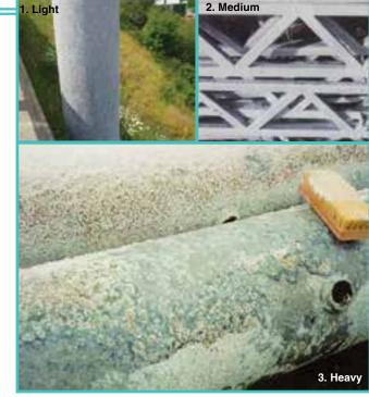
FIGURE 36: WET STORAGE STAIN [LIGHT (1) OR MEDIUM (2) IS ACCEPTABLE, HEAVY (3) IS REJECTABLE]
