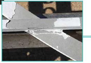
FIGURE 13: BLASTING DAMAGE (REJECTABLE
