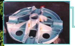
IGURE 29: SAND EMBEDDED IN CASTING (REJECTABLE)
