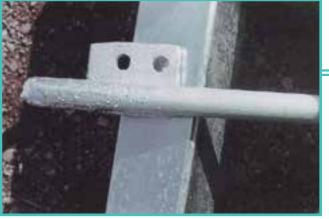
FIGURE 35: WELDING SPATTER (REJECTABLE)
