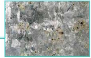
FIGURE 20: EXCESS ALUMINUM IN GALVANIZING BATH (REJECTABLE)
