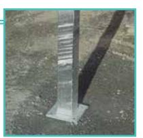
FIGURE 23: OXIDE LINES (ACCEPTABLE)
