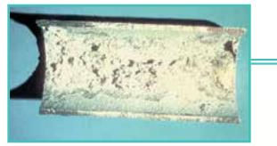
FIGURE 22: FLUX INCLUSIONS FROM INTERIOR OF PIPE (REJECTABLE)
