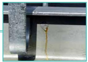
FIGURE 33: WEEPING WELD (ACCEPTABLE)
