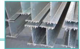
FIGURE 18: DRAINAGE SPIKES (ACCEPTABLE AFTER REMOVAL OR FILING)
