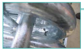
FIGURE 12: BARE SPOTS (REJECTABLE)
