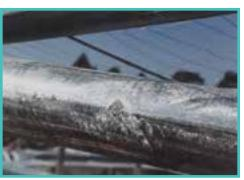
FIGURE 25: TOUCH MARKS (REJECTABLE)
