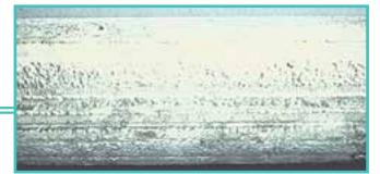
FIGURE 8: ROUGH COATING DUE TO PHOSPHOROUS LEVELS OVER 0.04% (ACCEPTABLE UNLESS HANDRAIL)
