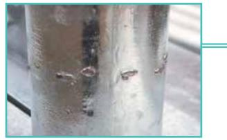
FIGURE 14: CHAIN AND WIRE MARKS (ACCEPTABLE UNLESS BARE STEEL IS EXPOSED)
