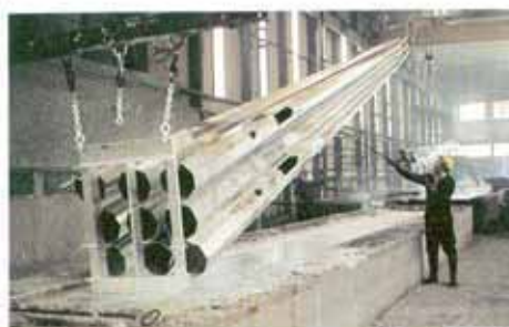
Galvanized lamp standards emerging from the bath of molten zinc.
