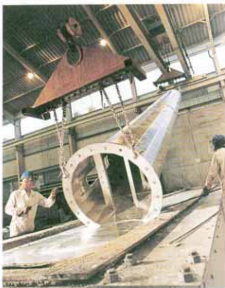
Large modular lighting poles are galvanized in sections for easier handling, shipping and on-site erection.
