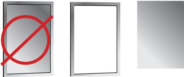
Figure 7: Galvanized thick frames separate from thin sheet/plate
