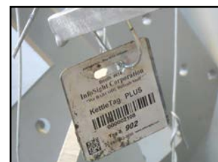
Figure 40: Metal barcode tags designed to withstand the HDG process can be easily removed.
