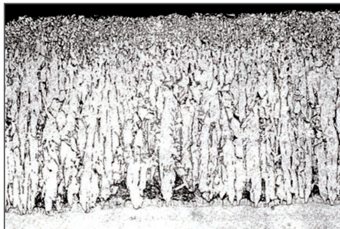
Figure 2: Atypical zinc-iron alloy layers
