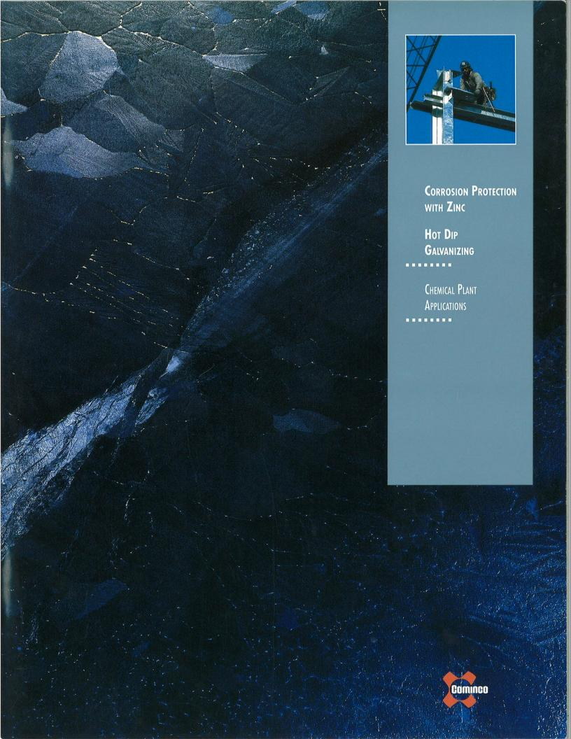
Cover: Close up of zinc coated steel showing familiar spangle resulting from hot dip galvanizing
