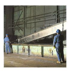
Galvanized structural beam emerging from a bath of molten zinc.
