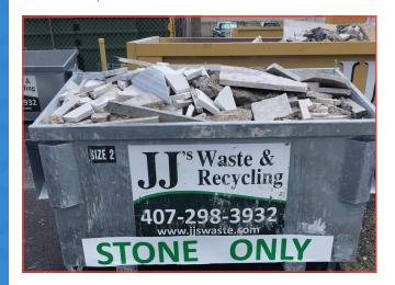
possibly as many as 15-20 years depending on the harshness of the environment, with the hotdip galvanized dumpsters. Based on average zinc coating thickness, the Time to First Maintenance is approximately 50 -75 years, even in the most extreme environments.
