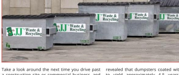
a construction site or commercial business, and you will likely see they have one thing in common; a trash dumpster that is rusting and falling apart because the paint coating could not protect it from its harsh and abusive environment. What makes JJ's Waste & Recycling so unique was their decision to hot-dip galvanize all of their industrial size trash dumpsters.
