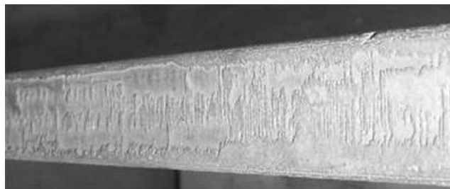
FIG. 5 Example of Hot-dip Galvanized Coating Appearance Formed Over Unprepared Flame-cut Edge on 1 in. Thick Steel
