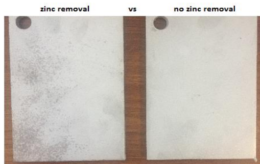
Figure 7: Example of Blasted Test Plates with Zinc Removal vs. No Zinc Removal
