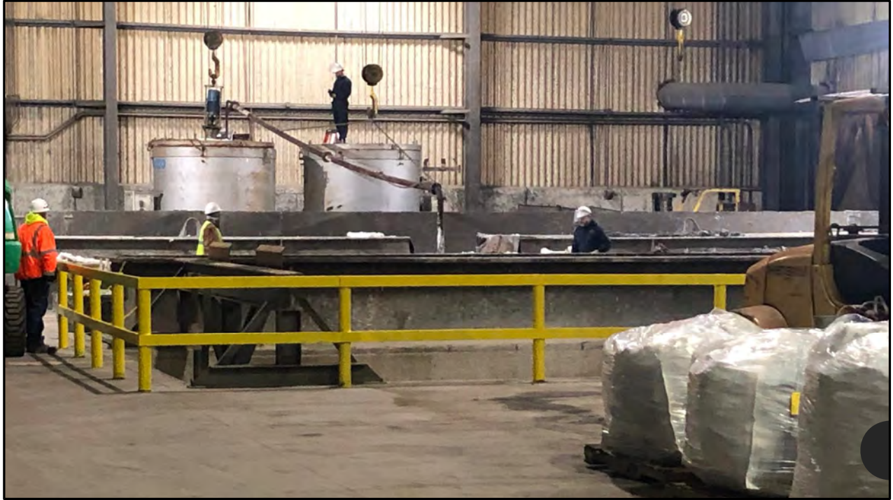
Another pump back from vessels with molten zinc.
