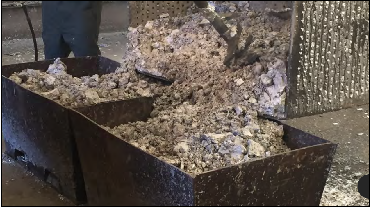
Picture of the nice grainy dross with zinc worked out. Barry Dugan says good dross only has 2 ½% to 3% iron in it.
