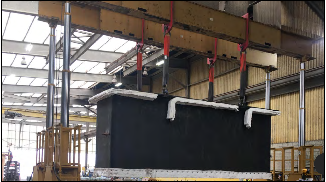
New kettle with wool installed getting ready to go into the hole.
