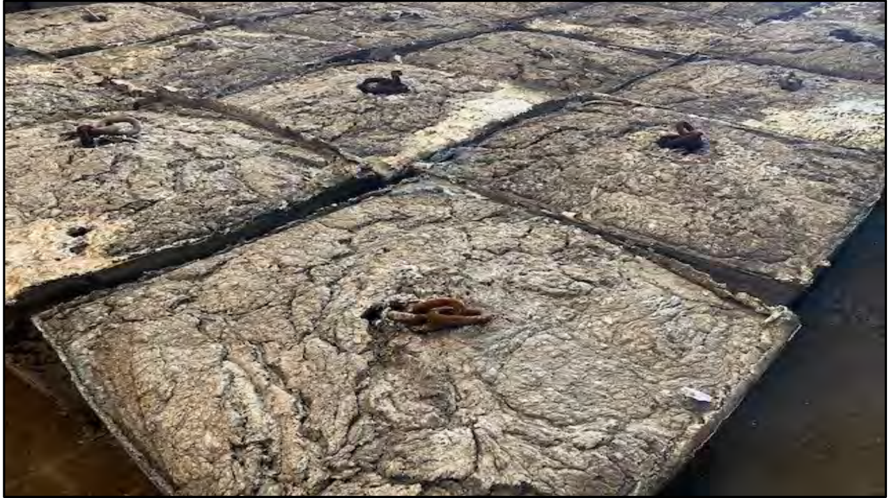
Zinc removed from pans and ready to stack in new kettle.
