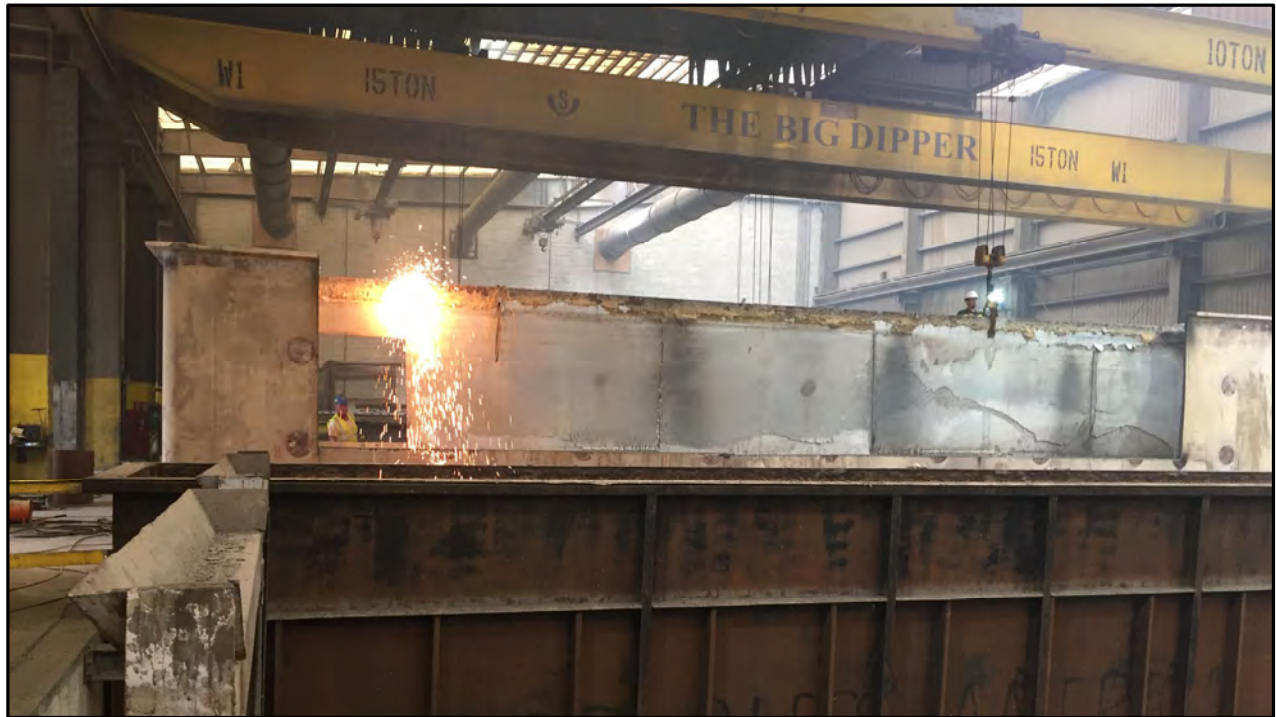
Cleaning up old kettle during meltdown period.
