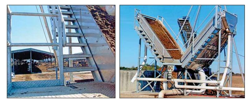
Dairy Production Systems milks 1,400 cows per day, and at this level of production, regular wash- downs of the milking parlor are required. The Static Screen Separator has helped turn waste disposal into profits. The separator takes manure and urine flushed from the milking parlor into holding tanks, and separates liquid from solids to the stack or lagoon to be recycled. It will produce 15 tons of solid waste per day, which can be spread or baled into compost.
