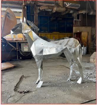
Alocal artist designed and fabricated the Horse Sculpture, a project that took hundreds of hours to fabricate. He chose to galvanize the piece after fabrication, and considering it is a hollow structure, the artist worked closely with the galvanizer to ensure the best result with the least modification to the piece. The galvanizer and artist collaborated to develop a plan that involved the least amount of venting and drainage holes – placed in discrete locations.
