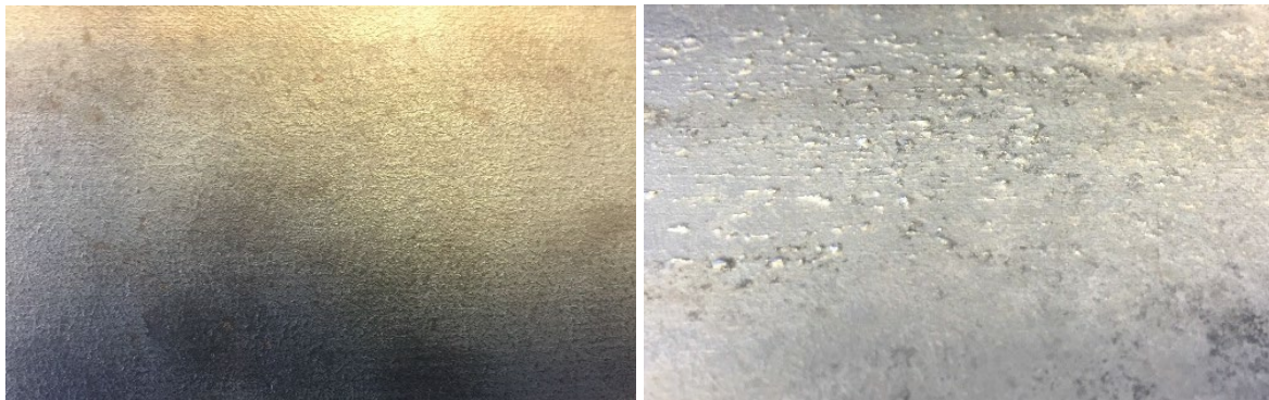
Figure 2: relatively smooth steel surface containing laps before galvanizing (left) and resulting coating formed after galvanizing (right)
