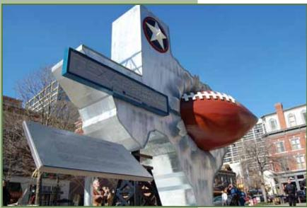
he "Cradle of Champions" sculpture was hot-dip galvanized for longevity of corrosion control, which was a concern due to the piece's prolonged exposure to the outdoor elements and environment. Galvanizing was also specified for its aesthetically pleasing appearance for this artistic endeavor.
